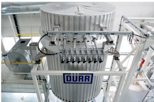
The organic paint particles in the saturated limestone powder, which serves as a binding material, are burnt in a fluidized bed furnace. The binding material can be re-used up to three times.
