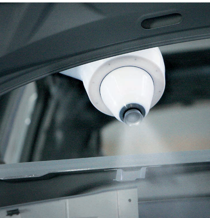
EcoBell3 Ci atomizer for interior painting shown in operation.
