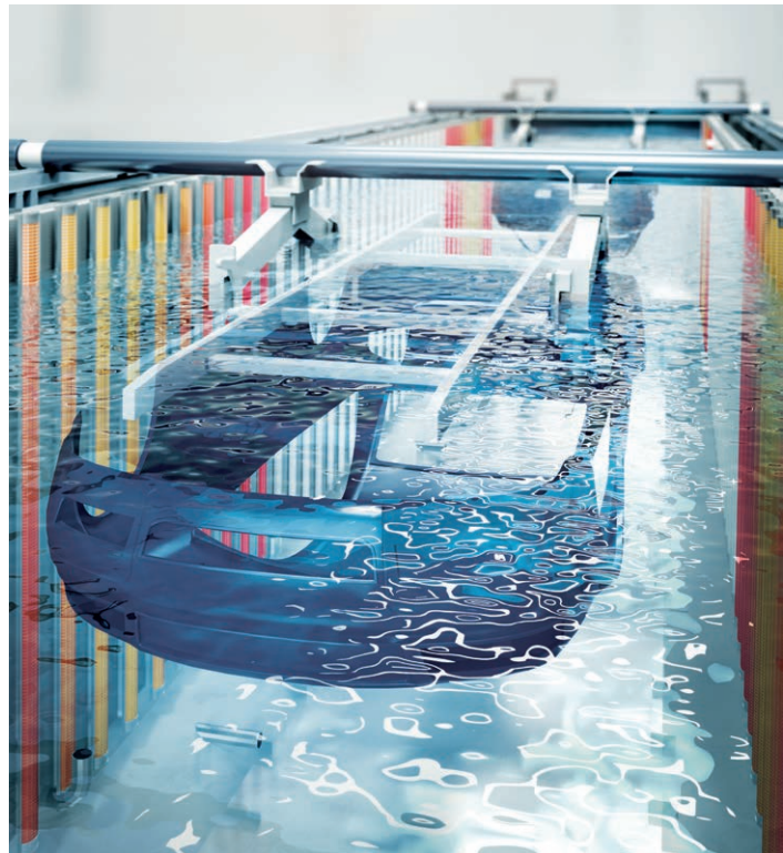
Targeted voltage supply in the cathodic dip bath with EcoDC MACS
