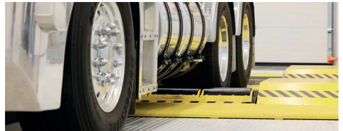
Example 3: 4 axles Front single roller movable, double roller and rear single roller movable together, rear single roller movable to double roller
