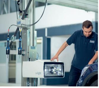
Light measuring device in operation
